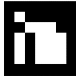
Figure 15: Example of ArUco marker
